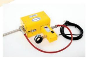
In conjunction with the heated filter probe, an automated self-regulated heated (180°C) Teflon tube may be used with the sampling line.
