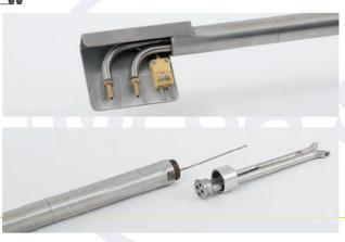
The PITOT "S" and PITOT "L" measuring tubes are used for measuring flow rate and air speed inside ducts. Attached to a sampling tube with nozzles and filter holder, they allow isokinetic sampling of emission dusts.
