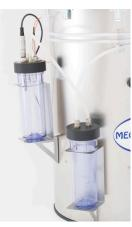
Optical sensor for reading oxygen in exhaust air.
